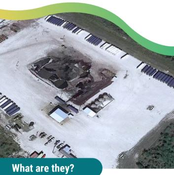
Surface waste disposal sites (SWDs) or "waste pits" are open air pits where oil and gas companies dump liquid and solid waste from the oilfield. Material disposed in waste pits may include drill cuttings, spent completion fluid, working fluids, and other oil and gas production waste. Some pits are located on well pads, and others combine waste from surrounding well sites.
